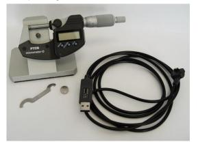
2. Unscrew the battery cover at the backside of the micrometer, remove the battery packaging and insert it with the positive terminal outward. After that properly mount the battery cover.
