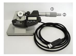
**9**. Data transfer to the PC by pressing the *DATA* button on the micrometer interface. The measured value is automatically transferred to the PC and is displayed in the opened program.
